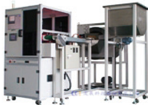
Fig. 5 — Glass disc-type AOI sorting machine with integral delicate feeding system.
